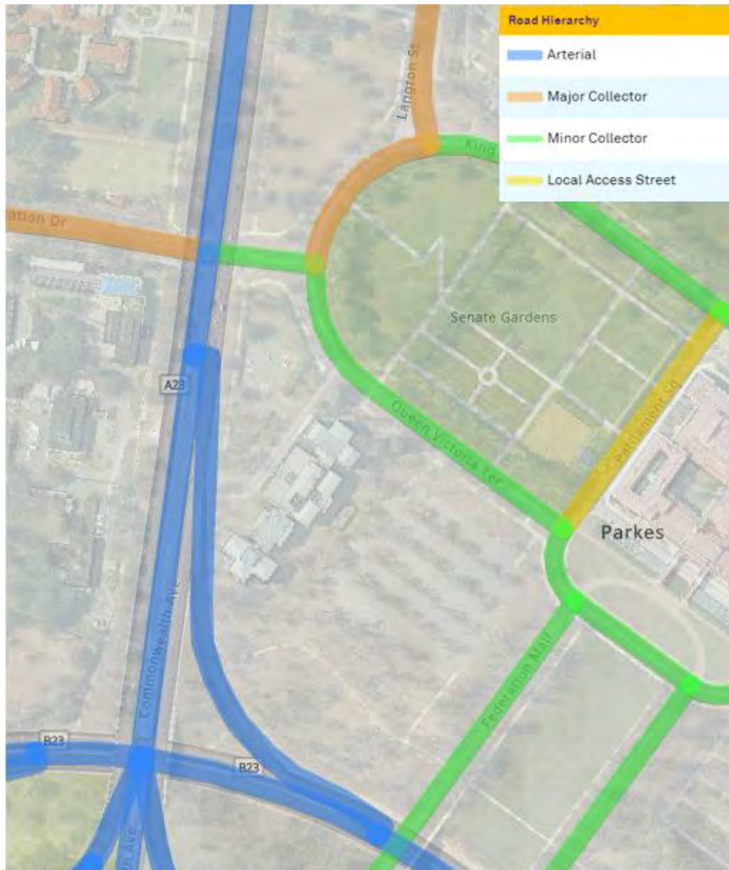
Figure 4-1 ACT Road Hierarchy Plan Around West Block (Source: Active Travel Practitioner's Tool)
