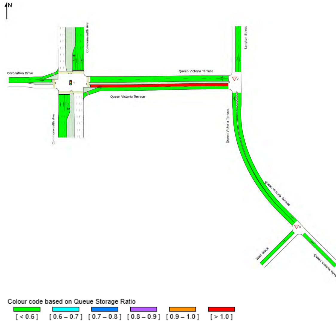
Figure 7-12 Operational Year PM 'With Development' Queue Length (95 th Percentile)
