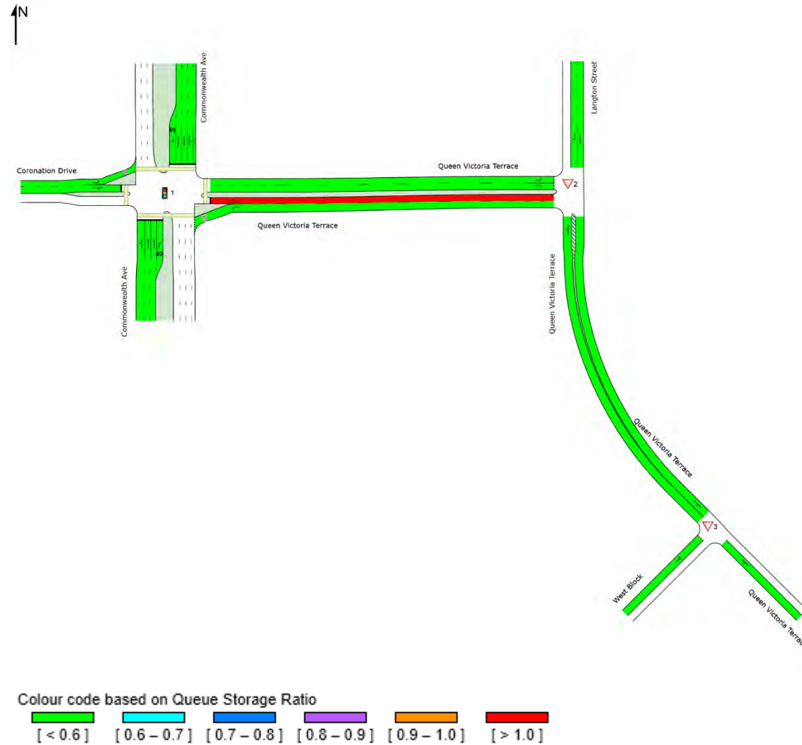
Figure 7-8 Operational Year PM 'Without Development' Queue Length (95 th Percentile)
