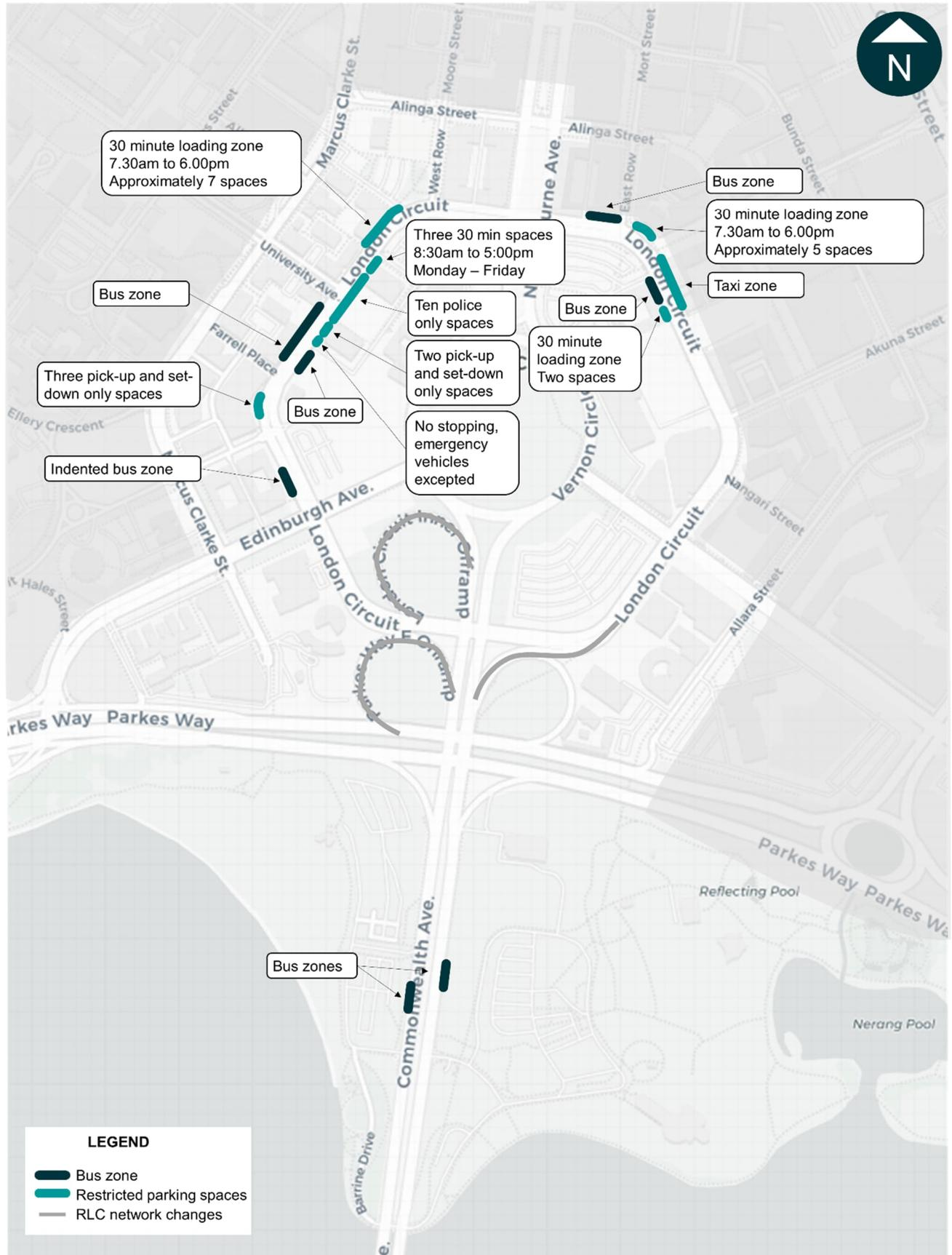
Figure 5-23 On-street parking and kerbside uses along the proposed alignment
