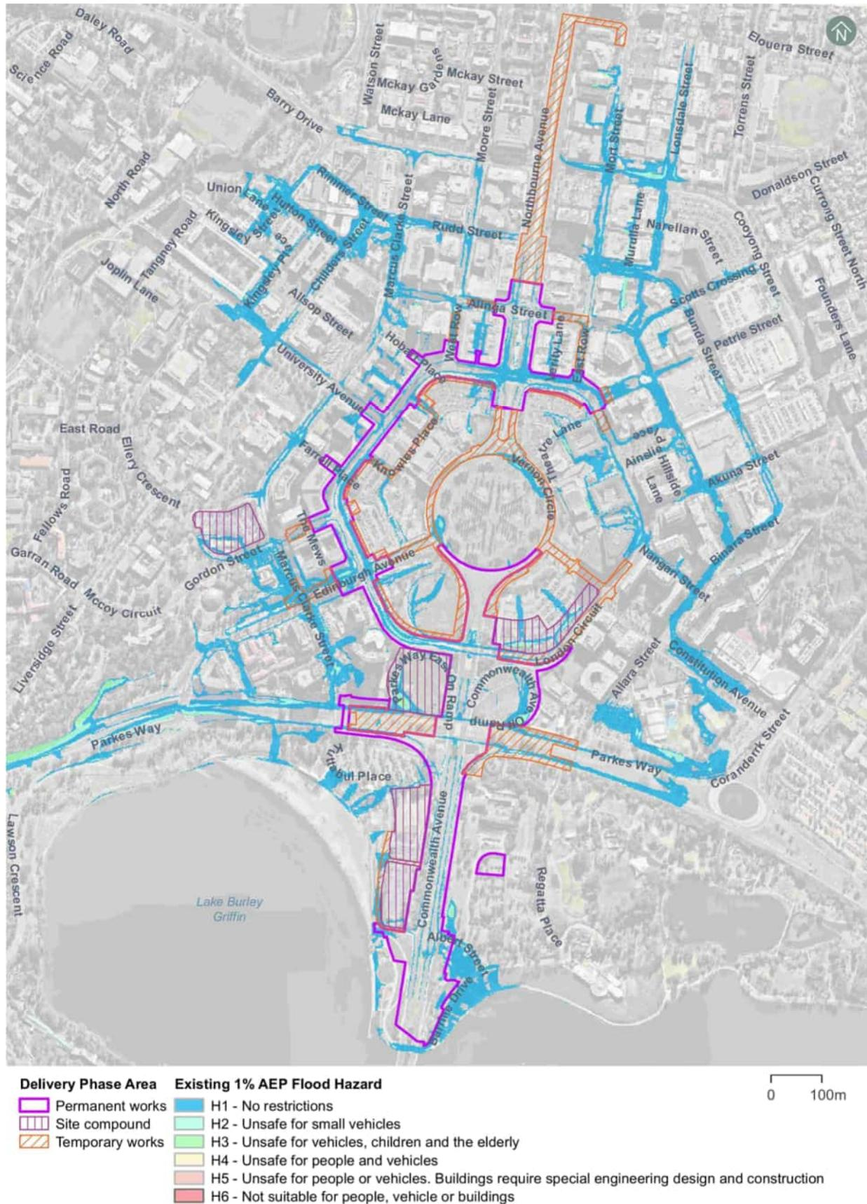
Figure 17-4 Existing conditions 1% AEP flood hazard (m)
