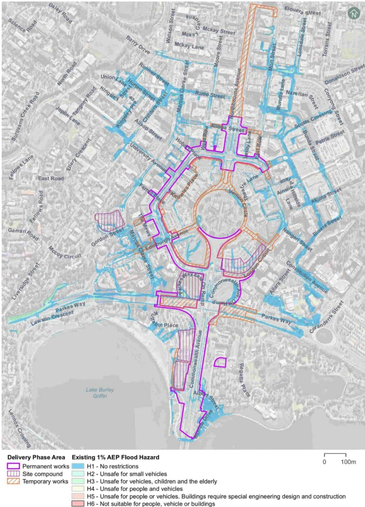
Figure 17-7 Flood hazard during operation of the Project (1% AEP event)
