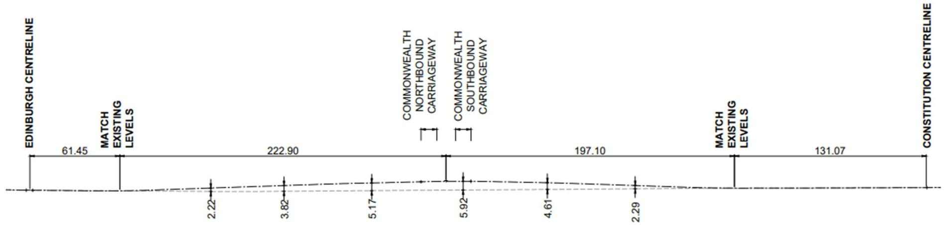
Figure 3-2 Indicative embankment vertical alignment along London Circuit
