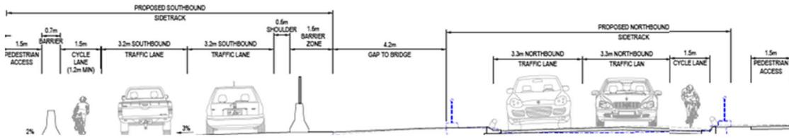
Figure 4-6 Indicative cross section through the temporary sidetrack and Commonwealth Avenue southbound carriageway during demolition of the Commonwealth Avenue northbound bridge
