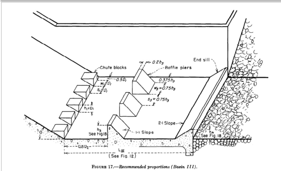
Types of stilling basin dissipators were progressively standardised based on experience, observations and model studies by the US Bureau of Reclamation (Akan and Iyer 2021). The SAF stilling basin, with chute blocks, baffle blocks and end sill became synonymous with the USBR Type III basin, although the term SAF basin continued to be used (Farhoudi, Sadat-Helbar and Aziz 2010).
