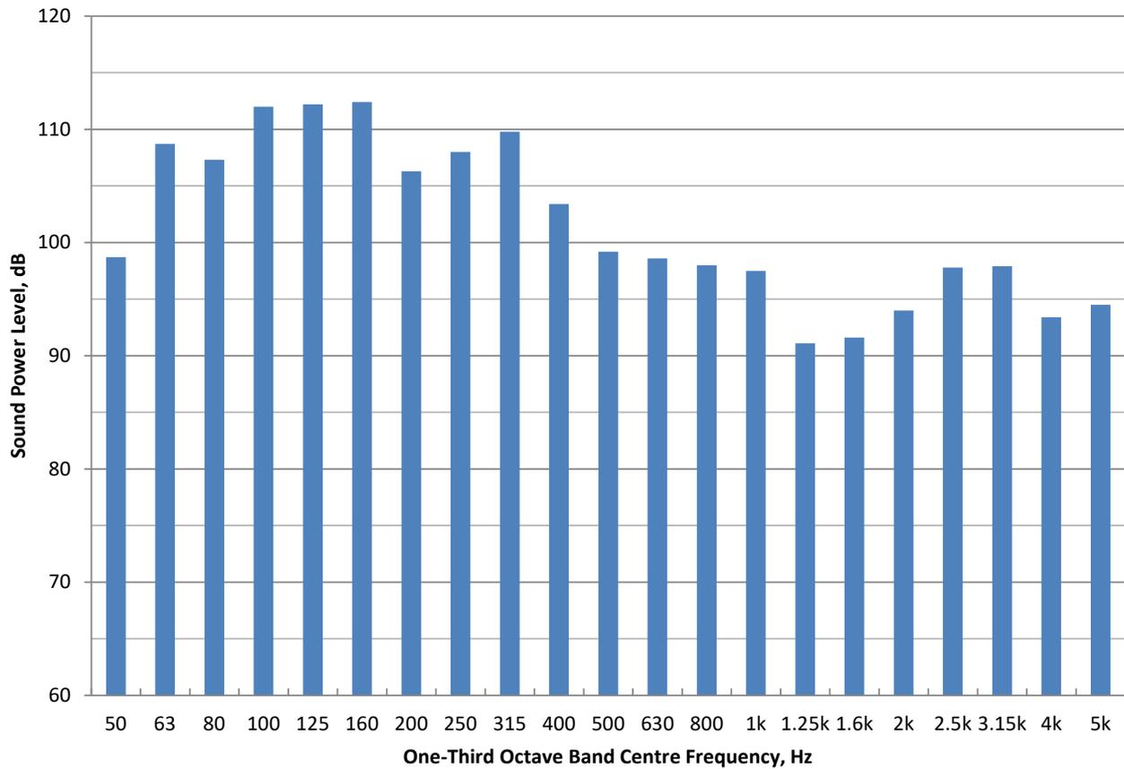
Figure 4.2 1/3 octave band sound power levels of rock drilling unit
