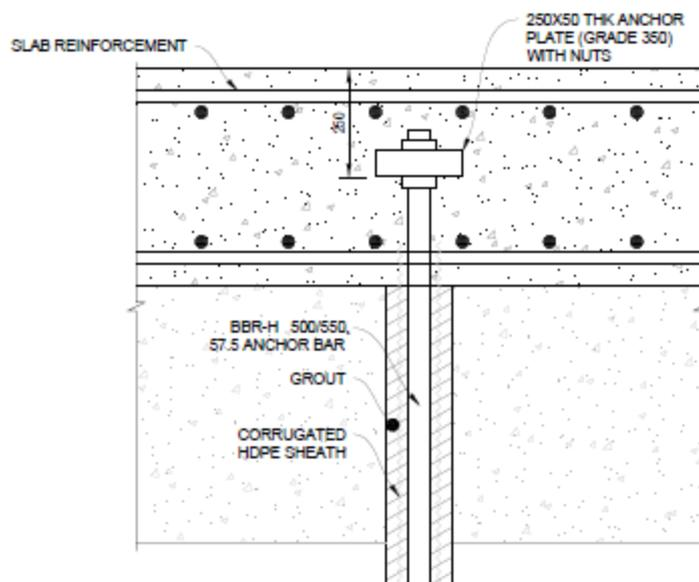
Figure 2.6 Anchor assembly and anchor head detail
