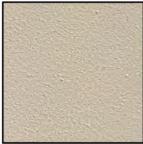
CON1 SCULPTED PRECAST CONCRETE WITH SAND OXIDE FINISH
