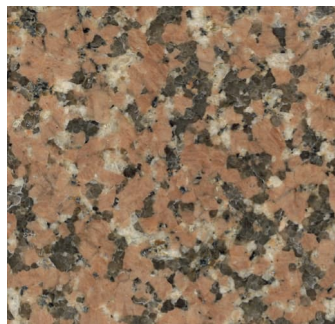
Figure 55: Tarana Pink Granite - original stone cladding.
