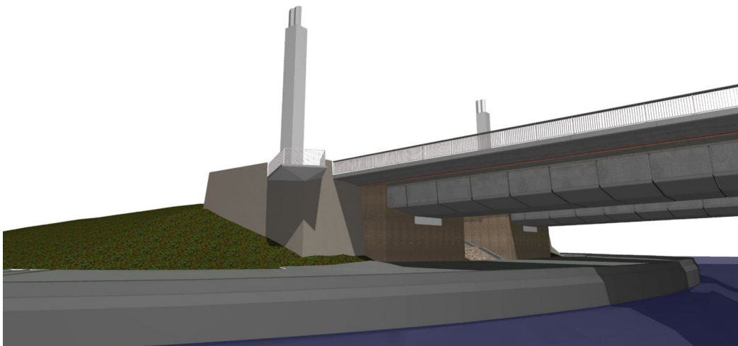
Figure 36: South abutment sketch perspective. Source: TZG Architects, June 2025.
