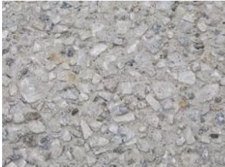
Figure 180: White precast concrete panel with exposed white Quartz aggregate.
