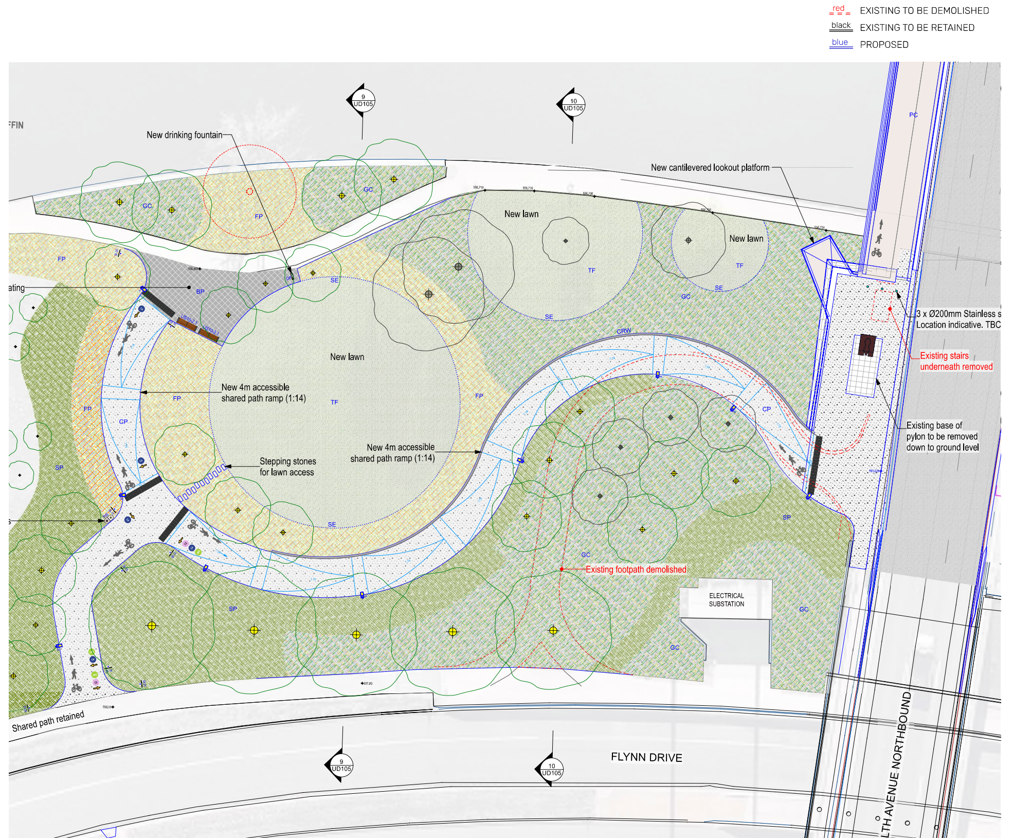
Figure 82: South-west approach (scale 1:400)
