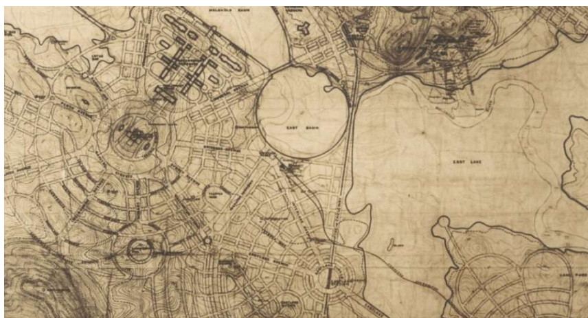
Figure 2. Walter Burley Griffin, 'Canberra, Plan of City and Environs,' 1918 (detail) showing the 'Eastlake Circle' rond point with Eastlake station at its centre on the main rail line of the Griffin Plan aligned north-south in a tunnel, or possibly a cutting, one of eight suburban stations on the line. Source: Nicholls Collection, National Library of Australia, 3665962.
