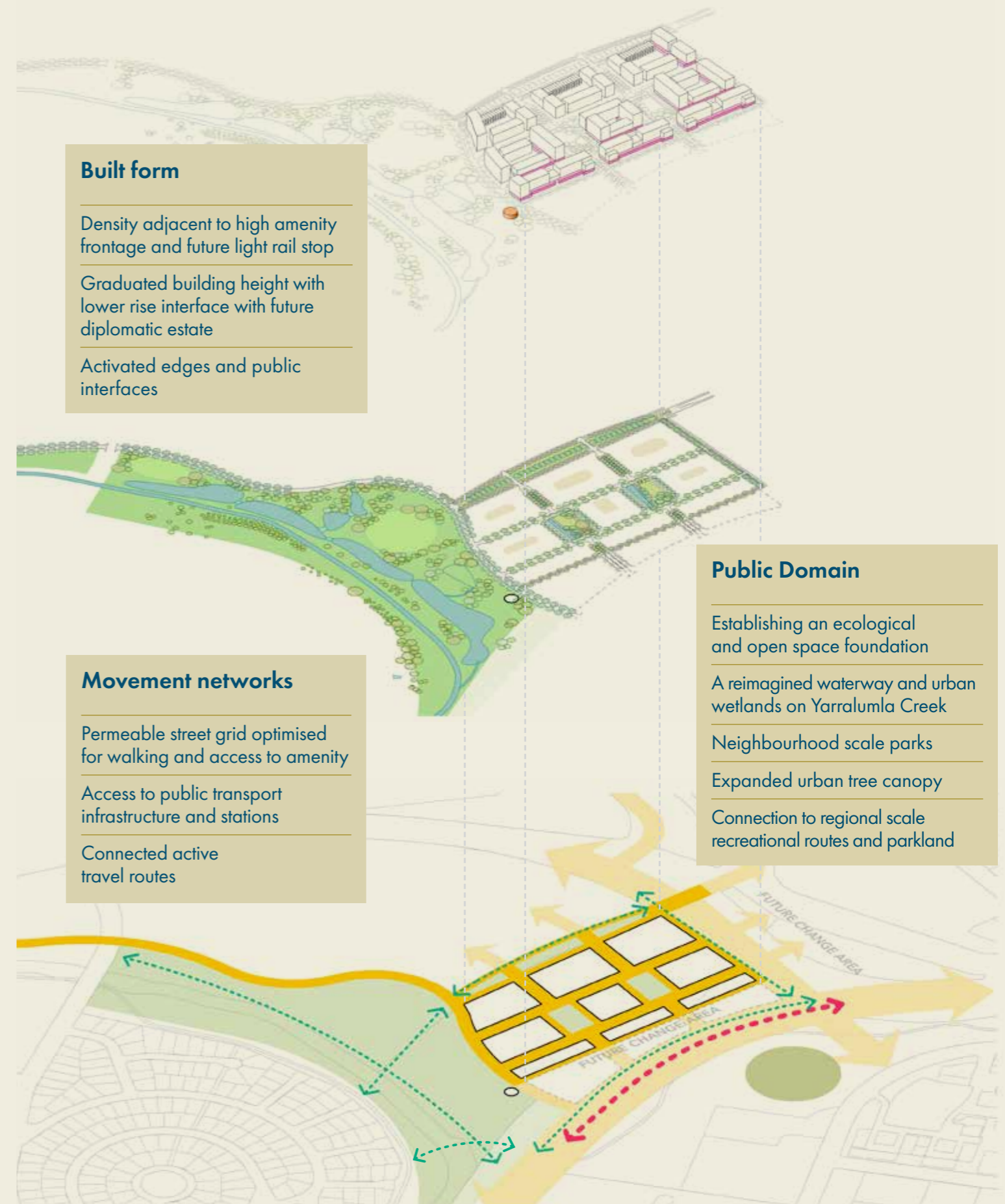
Figure 2: Indictive diagram - showing the superimposition of built form, the blue-green network and the movement networks planned for the North Curtin Residential Area.
