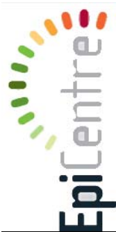
SIGN LOGO MATERIAL : ACRYLIC COLOURED 'ARC' FLUSH MOUNTED - BACK LIT FLUORESCENT LIGHTING ACRYLIC LETTERING RAISED 100mm - BACK LIT FLUORESCENT LIGHTING COLOUR : SEE ABOVE
