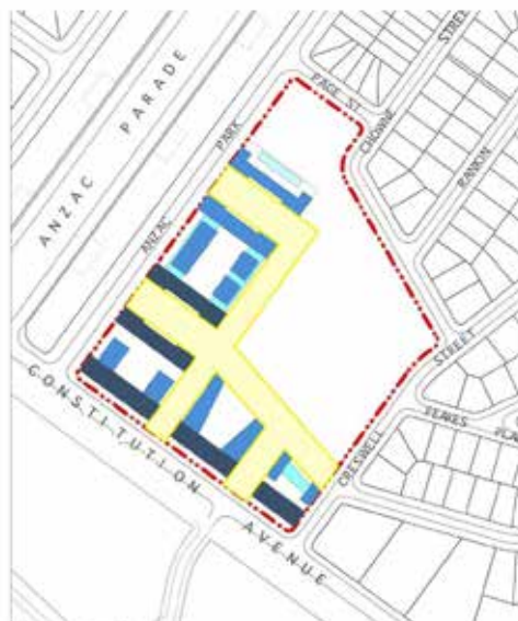
Figure 4 - Building Heights 10m maximum height 19m maximum height 13m maximum height 25m maximum height Street Reserve
