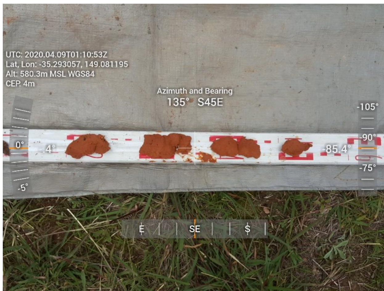
Soil texture assessment – soil ribbon average length of 65mm = Light Clay with Design Loading Rate (DLR) of 5mm/day
