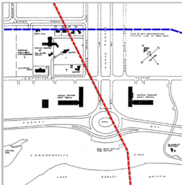
Figure 26. Plan of Anzac Parade showing 19 th Century road and c.1920 railway line
