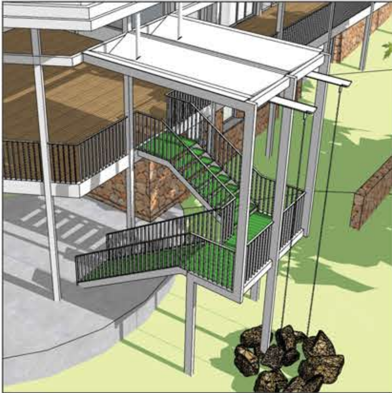
STAIR FROM GF TO LGF: (NORTH DECK, EAST SIDE) STAIR TREADS AND LANDINGS EQUAL TO TREADWELL FRP GRATEX STEP. STRINGERS 16THK X 200W STEEL FLATS WITH 50X10 FLAT WELDED TO TOP TO TAKE 50X10 BALUSTERS. HANDRAIL 50X16 FLAT. STAIR STRUCTURE 200X100X6 RHS. ROOF OVER STAIR FOLDED & WELDED 6MM THICK MILD STEEL PLATE TO FORM SPITTERS. PROVIDE 40X6MM GALVANISED CHAIN DPS DOWN TO SW SUMP. STEEL INFILL ROOF TO BE FABRICATED & HOT DIPPED GALVANISED. TACTILES AS REQUIRED.
