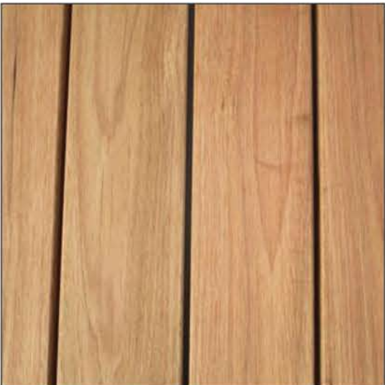
DECKING BOARDS: NOM 130W X 30THICK DAR KD BLACKBUTT, S/S SCREW FIX TO JOISTS ON DECKING PEDESTALS. OILED FINISH ALL ROUND BEFORE INSTALLATION. NOTE DECK SLABS TO BE FULLY WATERPROOFED WITH APPROPRIATE SHEET WATER PROOF MEMBRANE.
