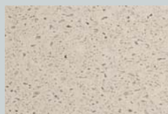
WT-1 - Coloured / textured concrete: Off white exposed aggregate polished precast
