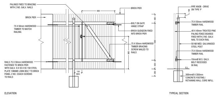
FENCE TYPE 2 & 3 - TIMBER PALING FENCE / GATE AND SCREEN
